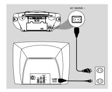
• After everything is connected properly, plug in the AC power cord to the power socket.
