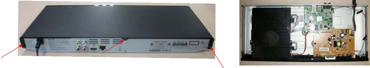
Step2: Dismantling Front Panel, the CD door should be removed first, then gently pull the Panel out from the set.
