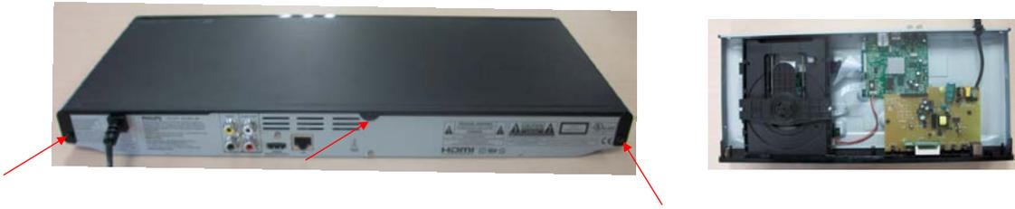
Step2: Dismantling Front Panel, the CD door should be removed first, then gently pull the Panel out from the set.
