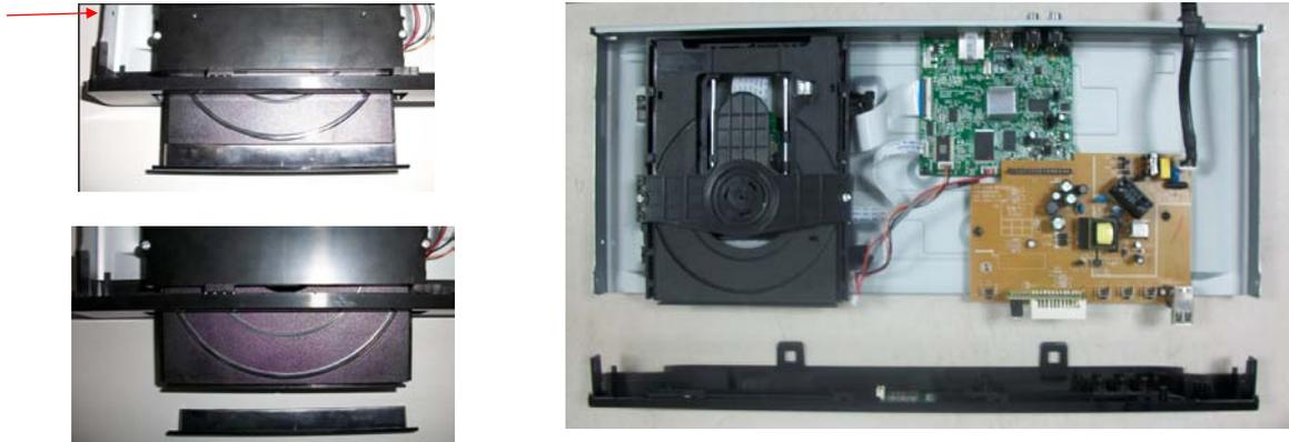
Step3: Remove the 9 screws on board to dismantle the DVD BOARD & PSU BOARD & DECK
