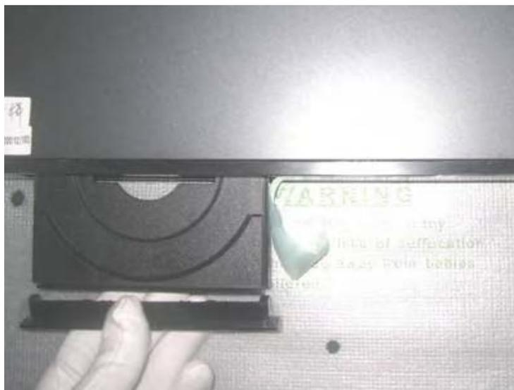
Please kindly note that dismantle the front door assembly carefully to avoid damage tray and the front door.
