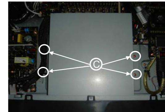
E. Loose 4pcs screws (3 x 16 BMTT) to remove the Power Board
