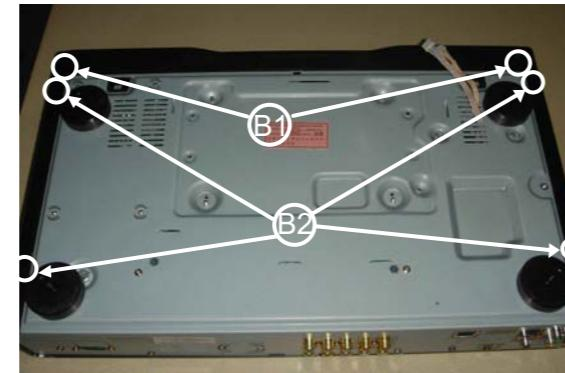
C. Loose 4pcs screws (3 x 5 BMTT) to remove the Blu-Ray Loader Driver Mechanism Cover
