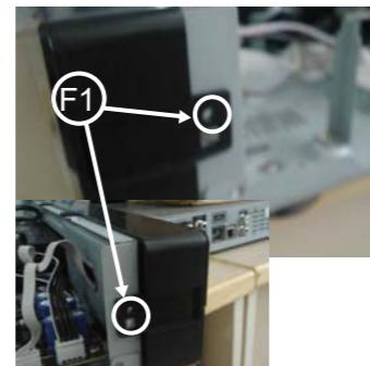
K. Loose 2pcs screws(2.6 x 8 BT) to remove the Display Board
