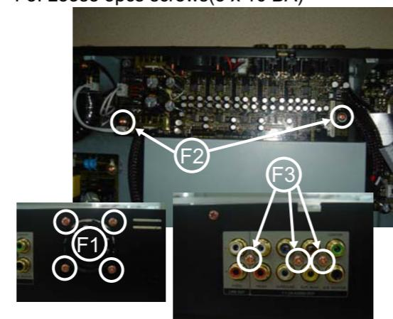
G. Loose 2pcs screws(3 x 5 BMTT) to remove the Power Transmit Board
