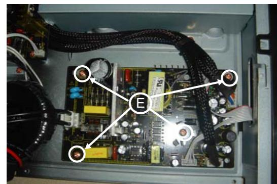
F. Remove the Output Board(Audio Board)
