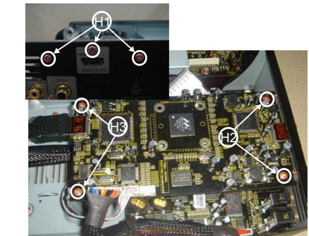
L. Loose 3pcs screws(2.6 x 8 BT) to remove the MCU Board
