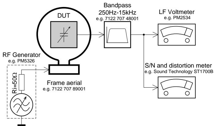
To avoid atmospheric interference all AM-measurements have to be carried out in a Faraday's cage.
