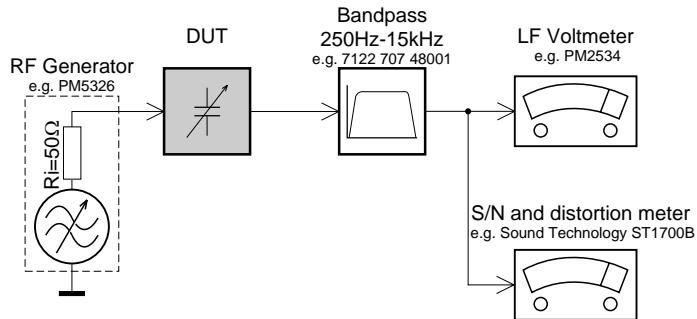
Use a bandpass filter to eliminate hum (50Hz, 100Hz) and disturbance from the pilottone (19kHz, 38kHz).
