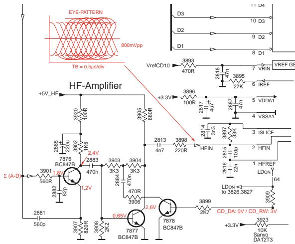
See below examples of the signal. Amplitude should read at least 700mVpp using SBC444A.
