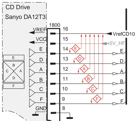
If one of the offsets is higher than  $\pm 10\text{mV}$  the CD drive has to be replaced. Otherwise replace the Signal Processor.
