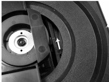
When a disc is loaded, unlock the tray by pushing the slide inwards by way of a screwdriver and pull tray outwards.
