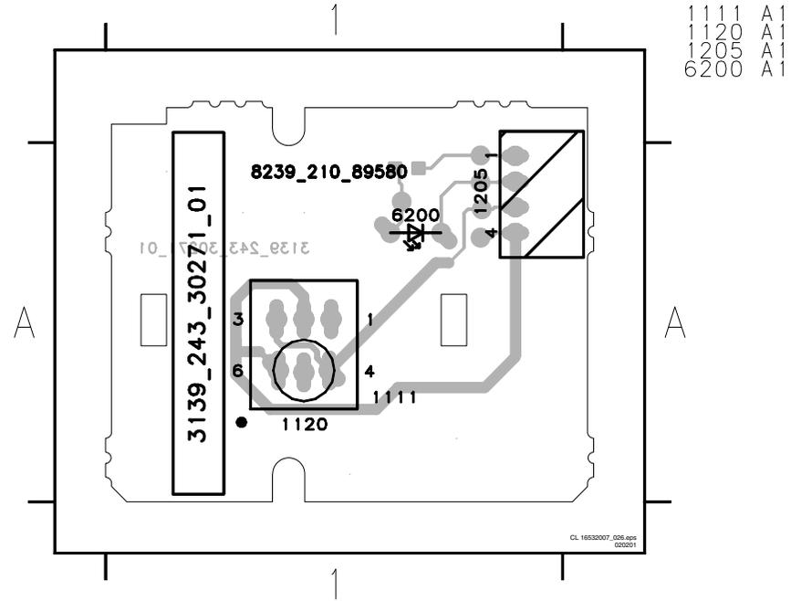
Layout Bare Board Standby (Component side)
