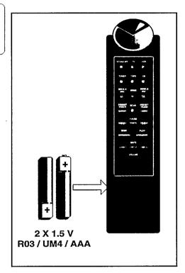
The remote control supplied can be used to operate all units in the system which are connected via the ESI sockets. In addition, it can be used to operate any other equipment that uses the RC-5 remote control system.
