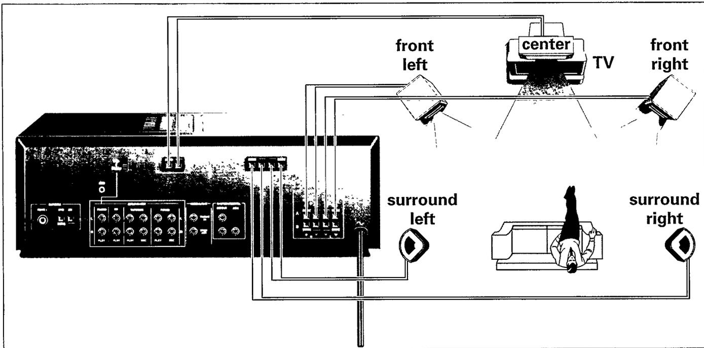
**Important ! Always switch off your amplifier/receiver before making any connections !**
