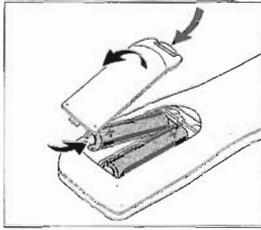
Remove batteries if they are flat or if the remote control is not going to be used for a long time.
