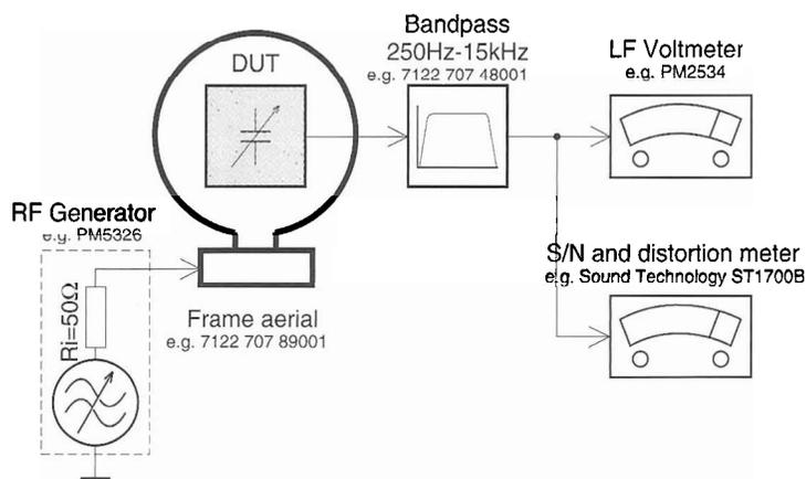
To avoid atmospheric interference all AM-measurements have to be carried out in a Faraday's cage.
