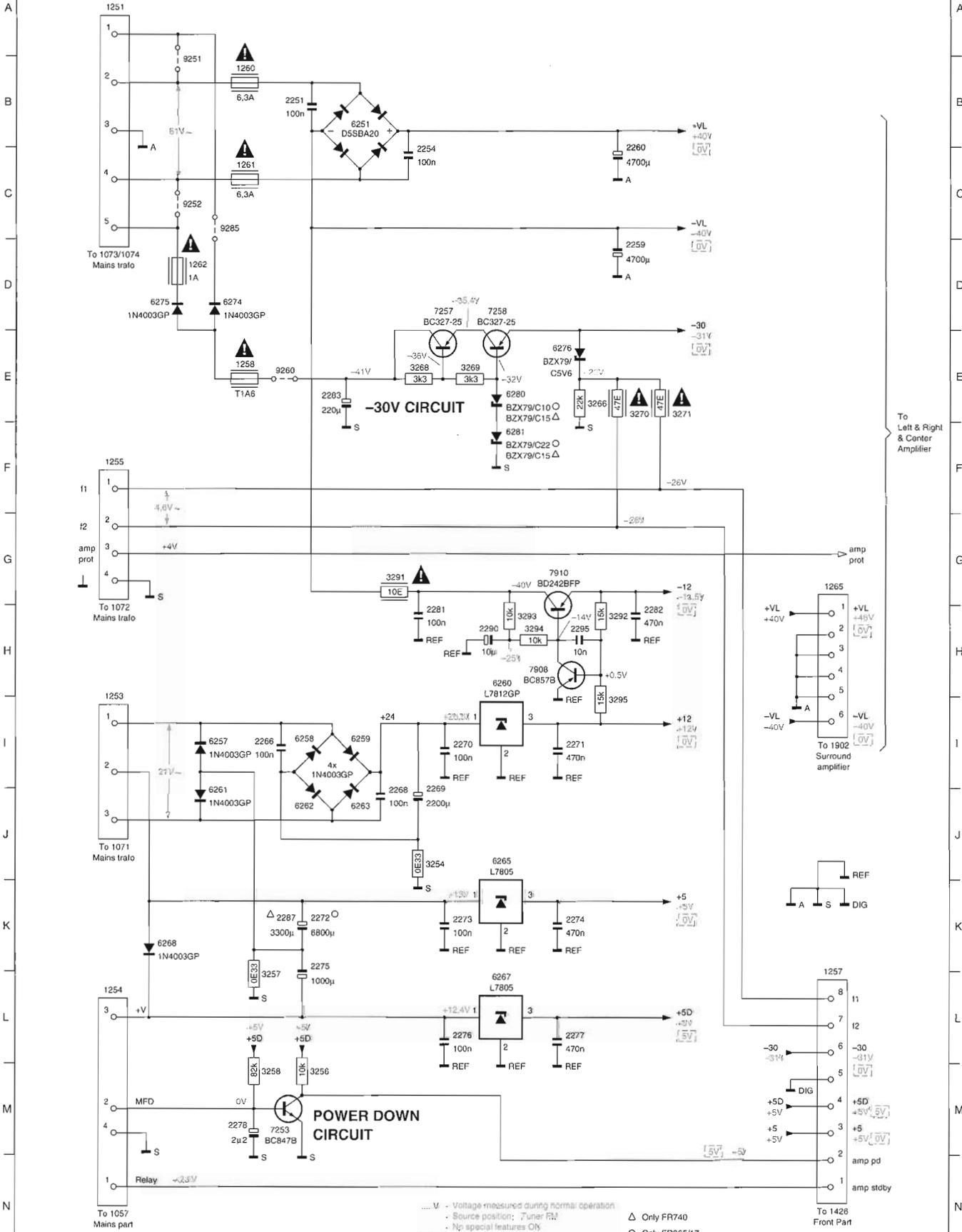
... V - Voltage measured during normal operation
