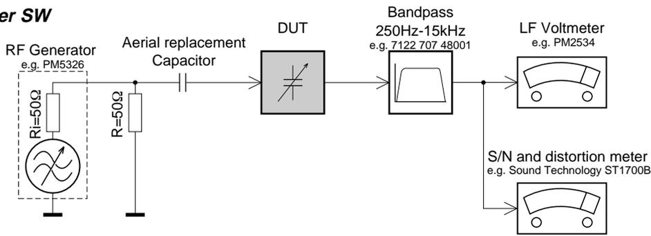
To avoid atmospheric interference all AM-measurements have to be carried out in a Faraday«s cage. Use a bandpass filter (or at least a high pass filter with 250Hz) to eliminate hum (50Hz, 100Hz).
