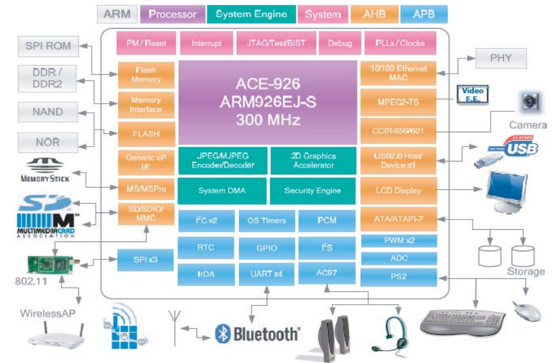
Figure 1 - VT8500 System Block Diagram
