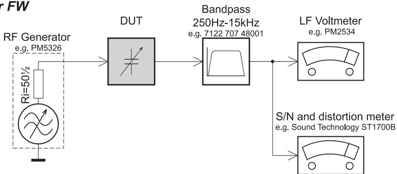
Use a bandpass filter to eliminate hum (50Hz, 100Hz) and disturbance from the pilottone (19kHz, 38kHz).
