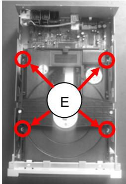
F. Loosen screws PHILIPS TORX T-10 1.5P 3.0X10.0 AB(4PCS), TORX STTP T-10 3.0X6.0 AB3(1PCS) to remove rear panel.
