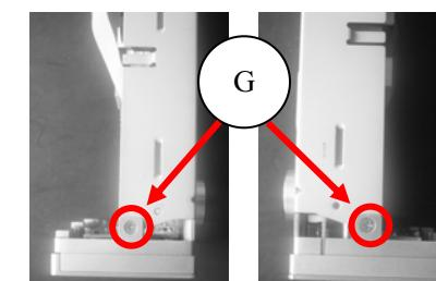
H. Loosen screws 3×5BM (3PCS) to remove AMP board.
