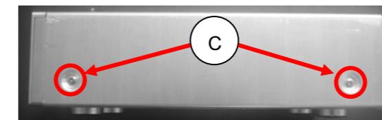
D. Loosen screws which located back of top cover TORX T-10 STTK 3.0×6.0NI(2PCS), and then reomoce top cover.
