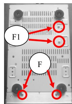
G. Loosen screws which located side cabinet 3×5FMTT(2PCS).
