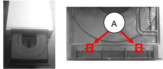
B. Loosen screws which located the left of cover TORX T-7 STTK 8010 3.0×6.0NI(2PCS)
