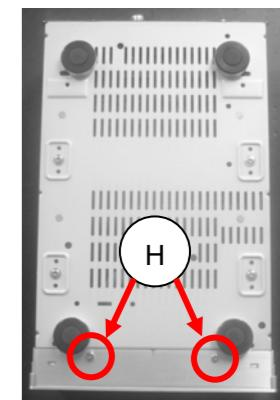
I. Loosen screws which located the side cabinet 3× 5FMTT(2PCS).
