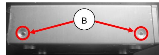
C. Loosen screws which located the right of cover TORX T-7 STTK 8010 3.0×6.0NI(2PCS).
