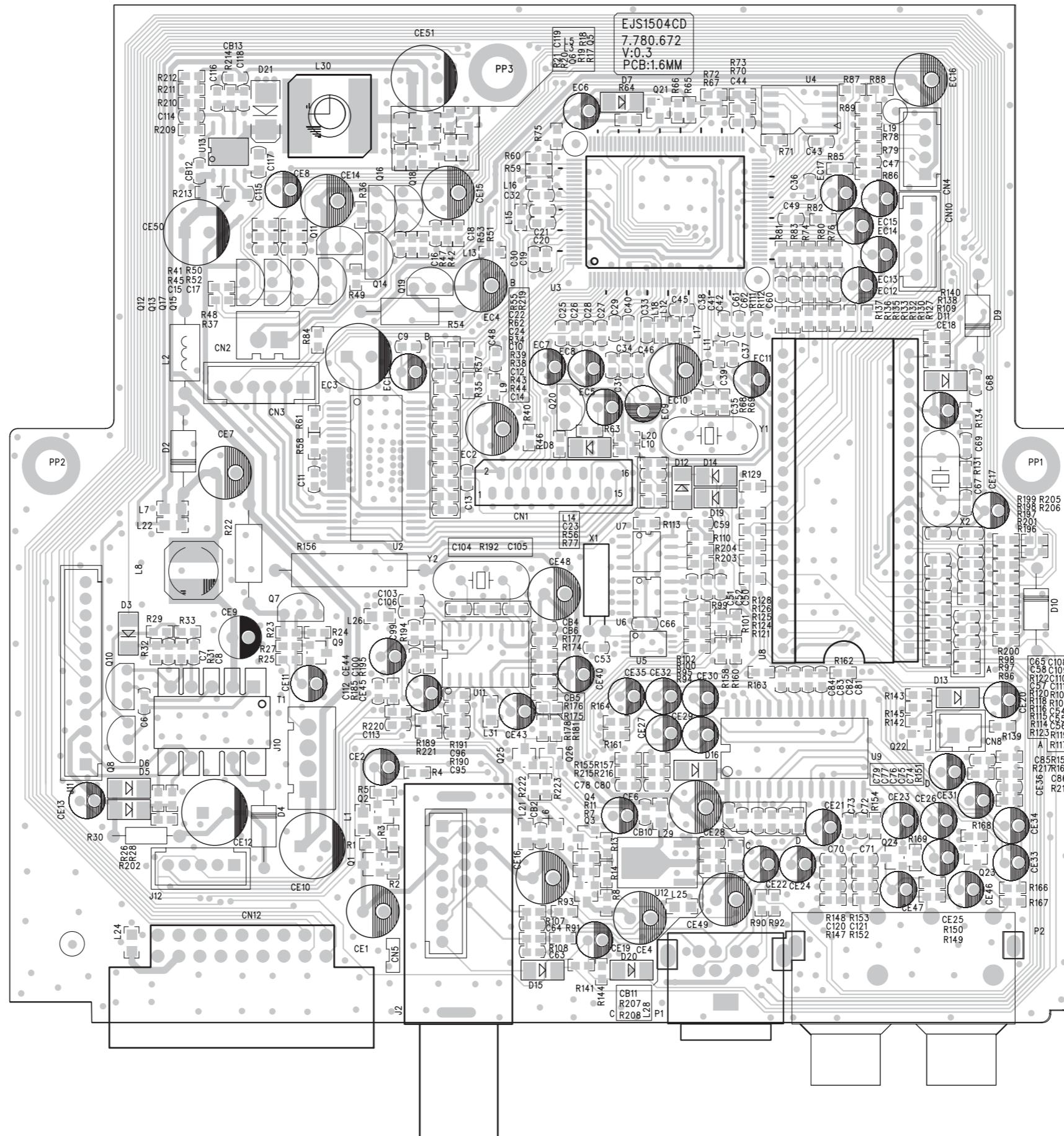
Decoder Board--Layout Diagram(Bottom)
