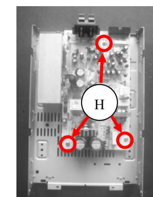
I. Loosen screws 2.6×8PA (4PCS) to remove volume board.
