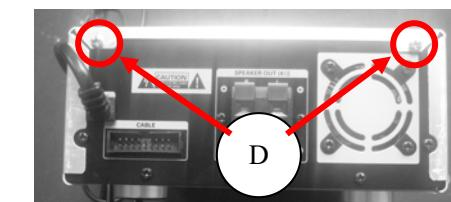
E. Loosen screws PHILIPS TORX T-10 1.5P 3.0X10.0 AB3(2PCS), TORX STTP T-10 3.0X6.0 AB3 (4PCS) to remove rear panel.
