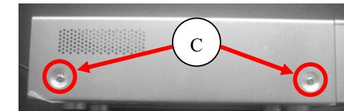
D. Loosen screws which located back of top cover TORX T-10 STTB 3.0X6.0 NI(2PCS).
