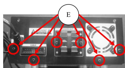
F. Loosen screws 3×5BMTT (2PCS) to remove bottom cover.
