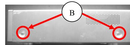
C. Loosen screws which located the left of top cover TORX T-7 STTK 8010 3.0X6.0 NI(2PCS).
