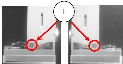
J. Loosen screws 2.6× 8PA(6PCS) to remove display board.
