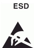
All ICs and many other semi-conductors are susceptible to electrostatic discharges (ESD). Careless handling during repair can reduce life drastically. When repairing, make sure that you are connected with the same potential as the mass of the set via a wrist wrap with resistance. Keep components and tools also at this potential.
