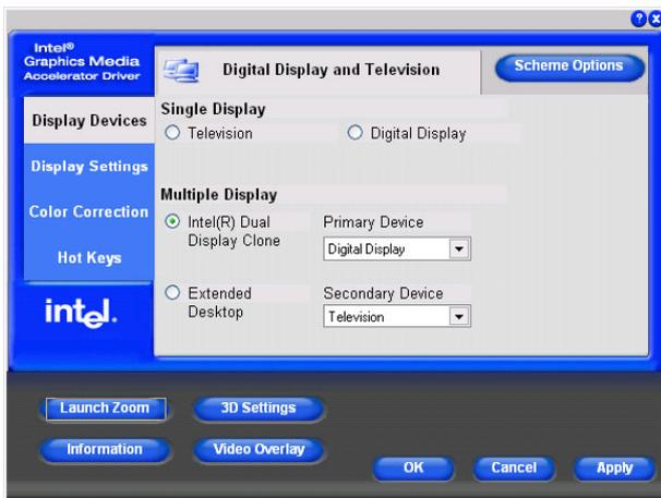
5. Switch you monitor and/or TV between the different inputs to check if the desktop can be seen on all four (Scart, DVI, VGA and S-Video) output modes.
