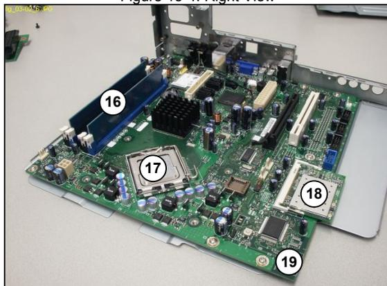
Figure 15-6: Motherboard subassembly
