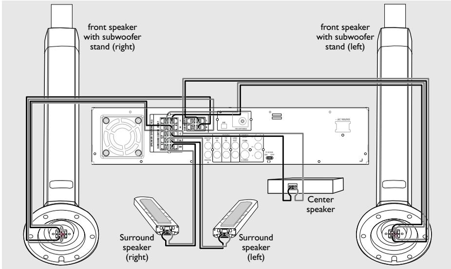
Connect the supplied speaker systems using the supplied speaker cables by matching the colors of the jacks and speaker cables. Fully insert the stripped portion of the speaker wire into the jacks.
