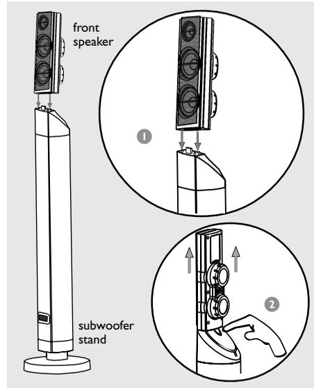
The connections between front speakers and DVD system are through the twin subwoofer stands.
