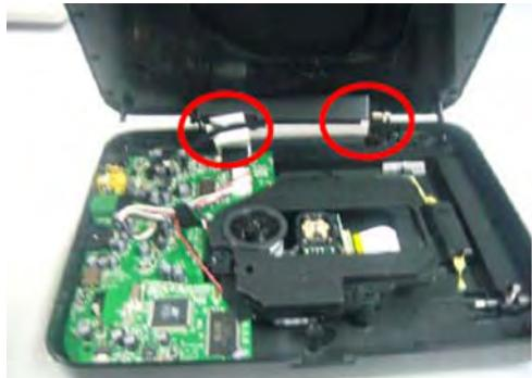
Step5: Remove screws to remove PCBAs
