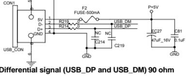
Differential signal (USB\_DP and USB\_DM) 90 ohm
