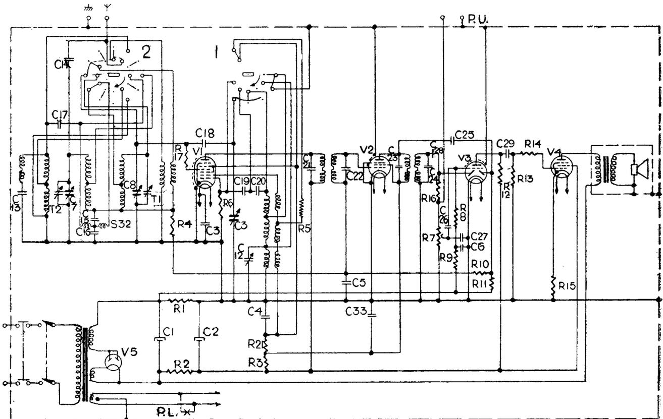
On the whole the circuit of the V5 follows the lines of any similar set constructed on orthodox lines. The I.F. transformers, however, are trimmed not by capacity but inductance. The switch diagrams are explained on the opposite page.
