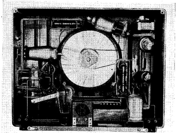
**CIRCUIT.**—A band-pass input circuit couples the aerial to V1, the frequency changer. The aerial is connected through a series condenser on long and medium waves and direct coupled on the short waveband.
