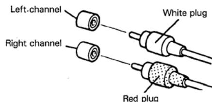
The INPUT/OUTPUT jacks of this unit are dull tinplated, for high audio quality.
