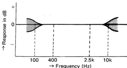
With BASS and TREBLE main controls set at 0dB, adjustment range of the sub-controls will be as shown by the shaded areas in the figure.
