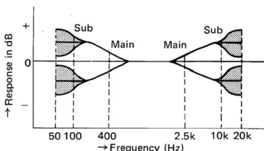
Adjusting first the main, then the sub controls can provide the range of adjustment shown by the shaded areas in the figure.
