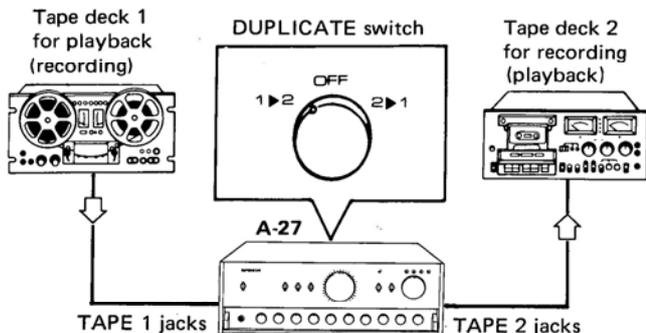
Set the DUPLICATE switch to 1 ▶ 2 when recording from tape deck 1 to tape deck 2.
