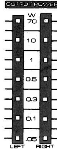
The output power indicators show the output level when speaker systems with a nominal impedance of 8 ohms have been connected to the rear panel speaker terminals. The output level (peak value) is indicated in watts by the scale units. Since a logarithmic compression scale is used, outputs ranging from the weak (0.05 W) to the strong (70 W) can be displayed without selecting the range.
