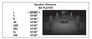
• The distance of all the speakers can be set to between 1 inch and 45 feet, in units of 1 inch.
