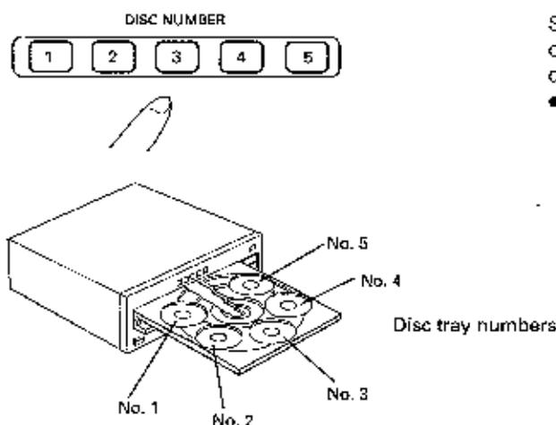
Select a disc using the DISC NUMBER buttons on the panel or remote control unit. The player searches for the specified disc and playback starts from the beginning of that disc.
