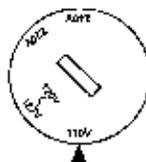
Set the selector so that arrow points to power voltage of your area (Figure shows arrow pointing to 110 volts.)
