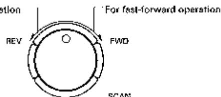
While rotating the SCAN control, playback advances or reverses at high speed. There are three scan modes which can be selected with rotational angles of the control.
