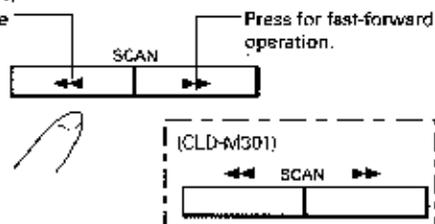
Normally Clear Scan is performed. To perform Low Scan and High Scan, press DISP on the remote control unit to display the screen and then press SCAN button. For about two seconds after the button is pressed, Low Scan is performed, after that, the unit enters High Scan.
