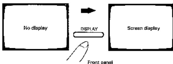
Information regarding the operations being carried out can be displayed on the screen of the monitor TV. When DISPLAY on the front panel or DISPLAY (CLD-M450/CLD-M401)/DISP (CLD-M301) on the remote control unit is pressed the first time, the screen display appears.
