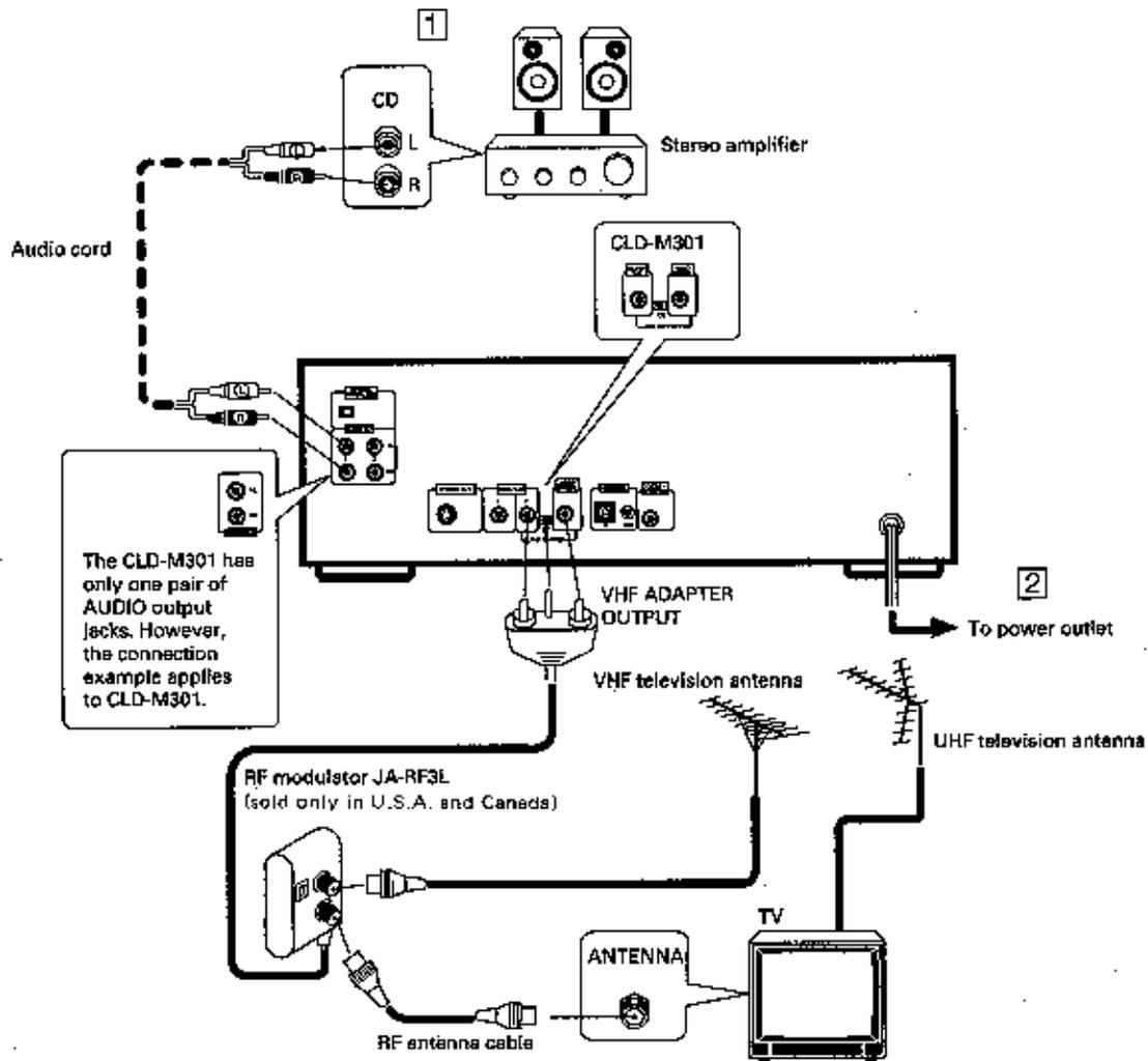
1. Detach the VHF antenna cable from the VHF antenna terminal of your TV set, and connect the cable to the VHF IN terminal of the RF modulator JA-RF3L.
