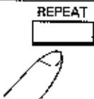
Press REPEAT on the remote control unit while the chapter/track to be repeated is playing. The REPEAT indicator lights on the display window of the front panel.
