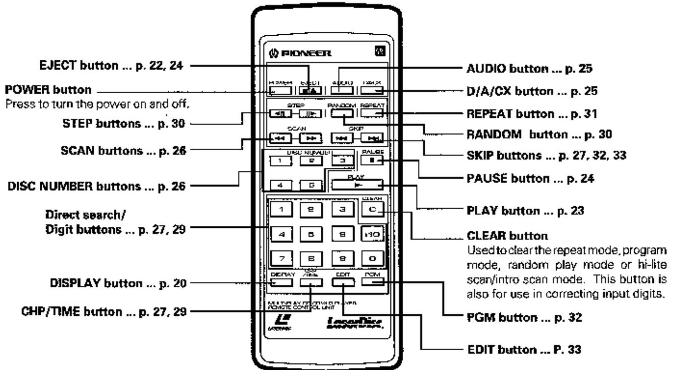
When operating the remote control unit, point the unit's infrared signal transmitter at the remote control receiver (REMOTE SENSOR) on the front panel of the player. The remote control unit can be used within a range of about 7 meters (23 feet) from the remote sensor, and within angles of up to about 30 degrees.
