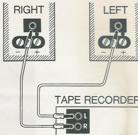
Connecting to a tape recorder-using cable with phone plugs on both ends.
