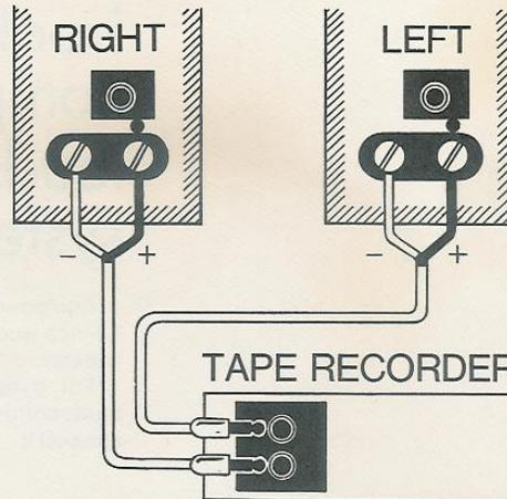
When using a connecting cable mounting a phone plug on one end and lugs on the other.
