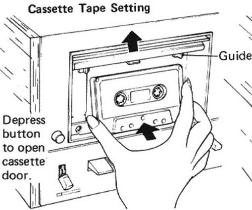
Align cassette between guides and insert with an upward motion.
