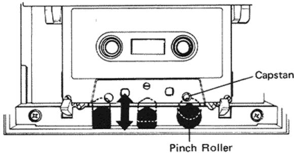
With PAUSE switch ON, pinch roller separates from capstan to temporarily stop tape motion; motor (capstan) and amplifier continue to operate."
