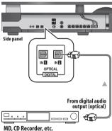
Connect the OPTICAL IN 2 jack on the side panel to the optical output of an external playback component. These include digital components such as an MD player, digital satellite, or a game system.
