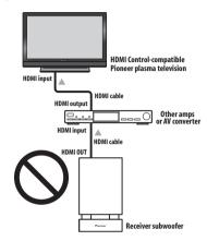
Only connect components you intend to use as a source to the HDMI input of this unit. Interrupting a direct connection with other amps or an AV converter (such as an HDMI switch) can cause operational errors.
