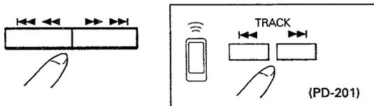
When  $\square \square \square \square$  is pressed once or a number of times, playback is advanced to the beginning of a track located after the track being played. The position of the located track corresponds to the number of times the button is pressed.
