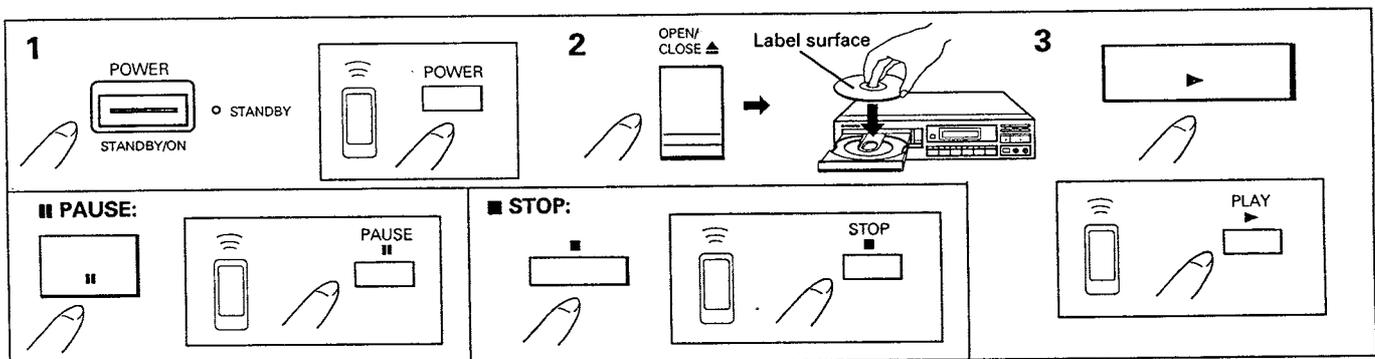
Operations indicated by the [ ] mark are performed with the remote control unit. (PD-201 only)
