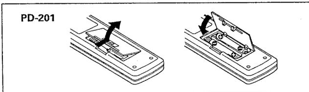
Open the lid of the battery compartment on the rear of the remote control unit, and insert the batteries, taking care to align the (+) and (-) polarities correctly.
