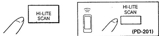
When HI-LITE SCAN is pressed during stop mode, playback starts from a point 1 minute after the beginning of the track, and each track is played for about 10 seconds. The SCAN indicator blinks during Hi-Lite scan mode.
