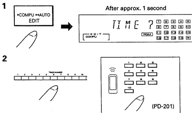
With this function, tracks are automatically programmed for both sides of the tape.
