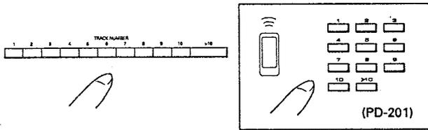
When the track No. is specified with the digit buttons, playback starts automatically from the beginning of the specified track.
