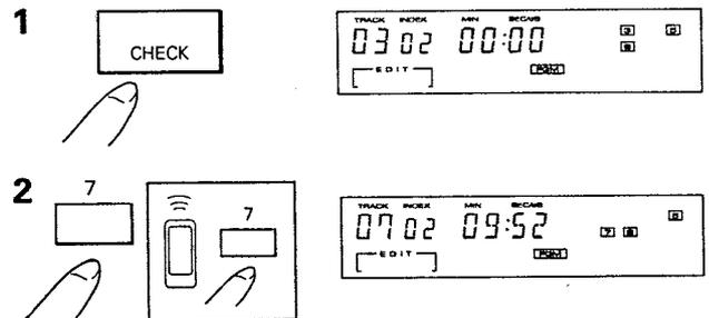
1. Press **CHECK** so that the program step to be corrected appears on the display.
