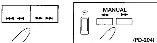
While ►►►► (or ►►►) is kept pressed, playback rapidly advances toward the end of the disc. When playback reaches the end of the disc, the player enters pause mode and "END" is displayed. While ◀◀◀◀ (or ◀◀◀) is kept pressed, playback rapidly reverses toward the beginning of the disc. When the desired passage is reached, release ►►►► (or ►►►) or ◀◀◀◀ (or ◀◀◀). The player enters original mode (playback or pause) where ►►►► (or ►►►) or ◀◀◀◀ (or ◀◀◀) is released.
