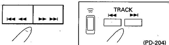
When ►►►► (or ►►►) is pressed once or a number of times, playback is advanced to the beginning of a track located after the track being played. The position of the located track corresponds to the number of times the button is pressed. When ◀◀◀◀ (or ◀◀◀) is pressed once, playback returns to the beginning of the track being played. When this button is pressed more than once, playback is returned to a track located before the track being played.
