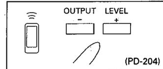
Press OUTPUT LEVEL "–" or "+" to adjust the output level.
