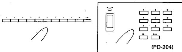
When the track No. is specified with the digit buttons, playback starts automatically from the beginning of the specified track. To specify track No. from 1 to 10, simply press the corresponding digit buttons (1-10). To specify track No. 11 or above, use >10.
