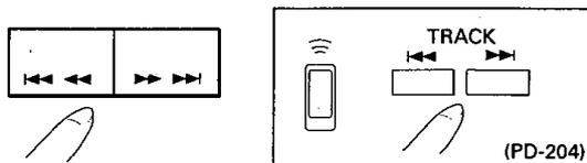
In the stop mode, pressing ►►►► (or ►►►) displays the playing time of each track starting from track No.1.
