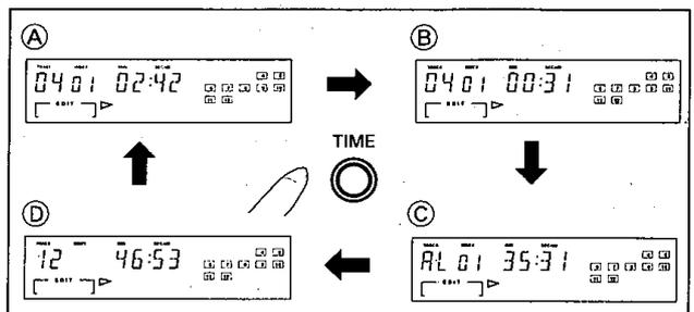
During playback, pressing the **TIME** button changes the time display in the following sequence: (A) Time (elapsed playback time of the track being played) → (B) Remain (remaining playback time of the track being played) → (C) AL Remain (remaining playback time from the playing point to the end of the disc) → (D) Total (total playback time of the disc).
