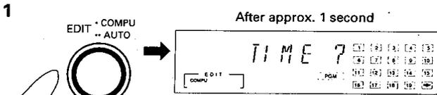
With this function, tracks are automatically programmed for both sides of the tape.
