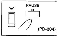
Inserting a pause in your program can be very useful when carrying out recording. Press **||** instead of entering a track number. "PA" appears on the display.
