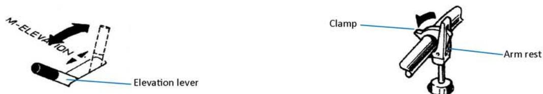
**ARM REST:** The arm rest supports the tonearm. As illustrated in the figure, use the clamp to keep the tonearm in place when you are not playing records.
