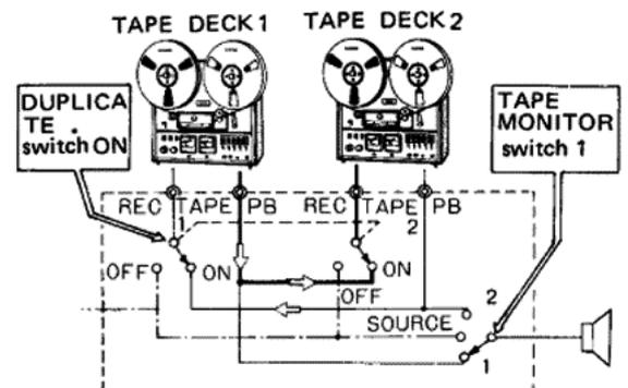
**Duplication:** Playback signal from tape deck 1 in the figure enters via TAPE 1 PB jacks, passes through DUPLICATE switch ON, and is recorded by tape deck 2. This can also be performed in reverse, ie: playback with tape deck 2 and record with tape deck 1.
