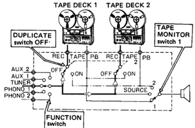
**Tape recording:** The input signal selected by the FUNCTION switch is always present at a fixed level at the TAPE 1 & 2 REC jacks. Monitoring can be performed at this time by setting the TAPE MONITOR switch to 1 or 2, according to the TAPE jacks being used for recording.
