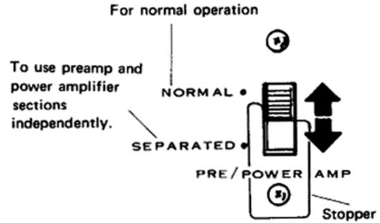
Switch for separating preamp and power amplifier sections.
