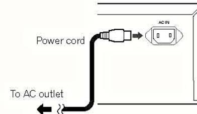
**1** Plug the supplied power cord into the AC IN socket on the rear panel of the unit.
