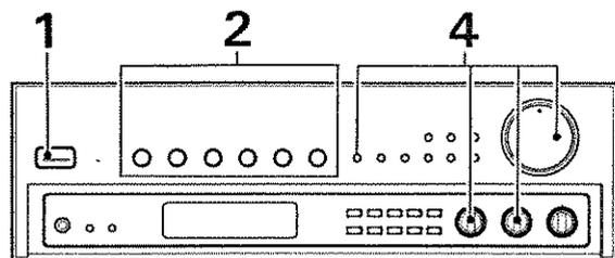
1. Press the **POWER** switch to the **ON** position. Also turn on the power to the stereo components you wish to use.
