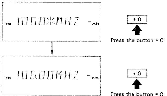
Once the station frequency has been input, the receiver tunes in that frequency. If the input frequency falls below the lower or higher limit of the receiver's receivable frequency range (FM: 87.5 MHz - 108 MHz; AM: 530 kHz - 1,700 kHz (10 kHz step), 531 kHz - 1,602 kHz (9kHz step) "LOWER" or "UPPER" is displayed, indicating that the frequency which has been input cannot be tuned in.
