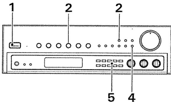
1. Press the POWER switch to the ON position.
