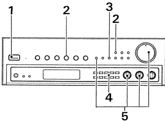
When you know the frequency of the desired station, the frequency can be input directly using the STATION CALL (number) buttons in the following way:
