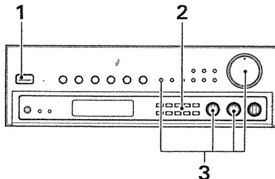
1. Press the POWER switch to the ON position.
