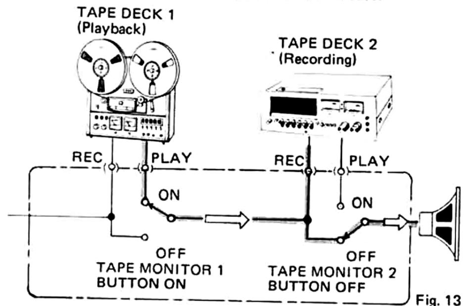
*Duplication: With the TAPE MONITOR 1 button set to ON, the TAPE 1 deck playback signal proceeds in the arrow direction where it can be recorded by TAPE 2 deck. While listening to the sound from the speakers, operate TAPE 2 deck controls (PAUSE button, etc.) in order to record only the desired signal.*
