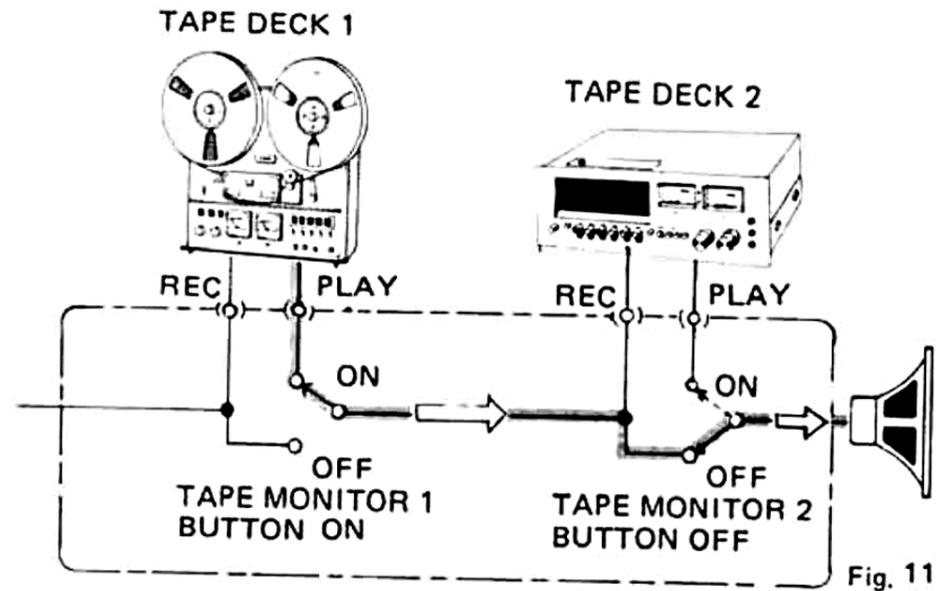
*Tape Playback: TAPE MONITOR 2 button must be OFF, and TAPE MONITOR 1 button ON to play tape on TAPE 1 deck. Signal enters PLAY jacks and proceeds in arrow direction to be amplified and transferred to the speakers. Set TAPE MONITOR 2 button to ON to play tape with TAPE 2 deck.*
