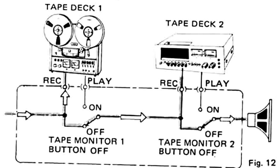
*Tape Recording: Signal selected by the FUNCTION switch appears at the TAPE 1 REC jacks. If TAPE MONITOR 1 button is set to OFF, the same signal also appears at the TAPE 2 REC jacks. Simultaneous recording with 2 tape decks can be performed in this case.*
