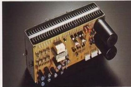
uses thinly-sliced metal fins on a lightweight but solid frame to provide as much as 50% better heat dissipation than in conventional types.
