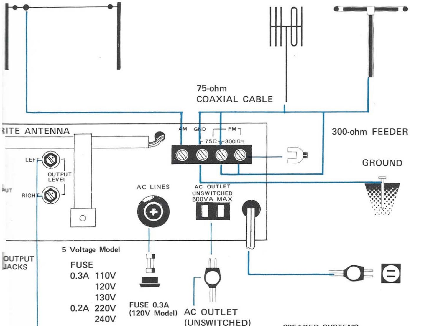
FM/AM Output level controls to increase the output level, turn to the right.
