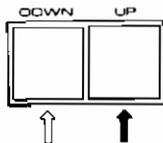
If the frequency of the broadcasting station to be tuned in is lower than the frequency on the display, depress the DOWN switch lightly. If it is higher, depress the UP switch.
