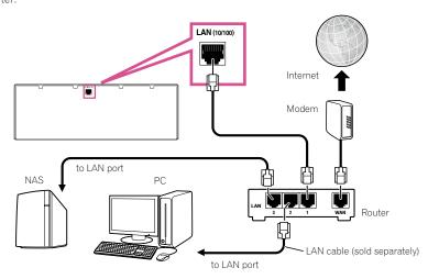
Connect the LAN terminal on this receiver to the LAN terminal on your router (with or without the built-in DHCP server function) with a straight LAN cable (CAT 5 or higher).
