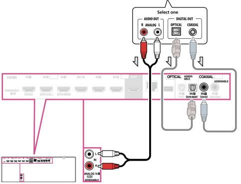
• If your turntable has line-level outputs (i.e., it has a built-in phono pre-amp), connect it to the **ANALOG IN 1** (CD) inputs instead.
