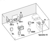
With these connections you can simultaneously enjoy 5.2-channel surround sound in the main zone with stereo playback of the same sound on the B speakers. The same connections also allow for 7.2-channel surround sound in the main zone when not using the B speakers.
