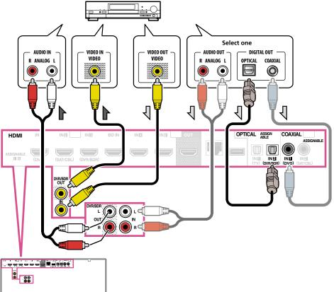
• In order to record, you must connect the analog audio cables (the digital connection is for playback only) (page <u>64</u>).
