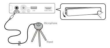
If you have a tripod, use it to place the microphone so that it's about ear level at your normal listening position. If you do not have a tripod, use some other object to install the microphone.
