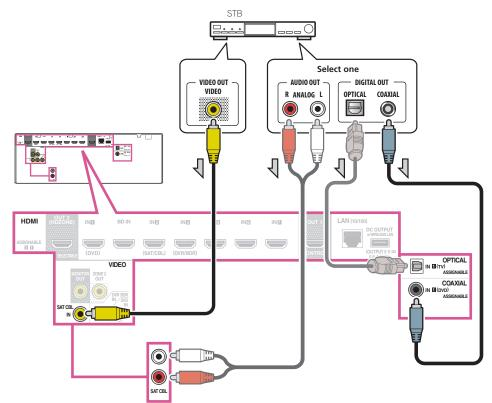
If your set-top box is equipped with an HDMI output terminal, we recommend connecting it to the receiver's HDMI SAT/CBL IN terminal. When doing so, also connect the receiver and TV by HDMI (see <u>Connecting using HDMI</u> on page 24).
