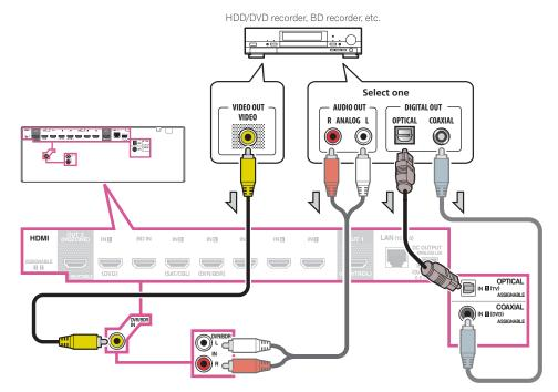
If your HDD/DVD recorder, BD recorder, etc., is equipped with an HDMI output terminal, we recommend connecting it to the receiver's HDMI DVR/BDR IN terminal. When doing so, also connect the receiver and TV by HDMI (see <u>Connecting using HDMI</u> on <u>page 24</u>).
