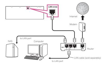
Connect the LAN terminal on this receiver to the LAN terminal on your router (with or without the built-in DHCP server function) with a straight LAN cable (CAT 5 or higher).
