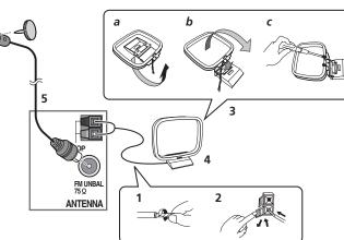
1 Pull off the protective shields of both AM antenna wires.
