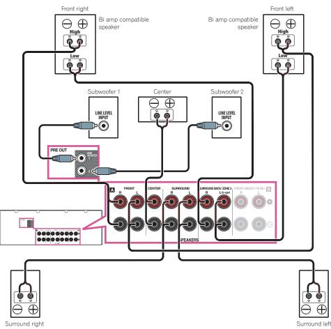
Most speakers with both High and Low terminals have two metal plates that connect the High to the Low
