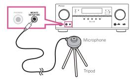
If you have a tripod, use it to place the microphone so that it's about ear level at your normal listening position. If you do not have a tripod, use some other object to install the microphone.
