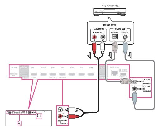
• If your turntable has line-level outputs (i.e., it has a built-in phono pre-amp), connect it to the **ANALOG IN 1** (CD) inputs instead.
