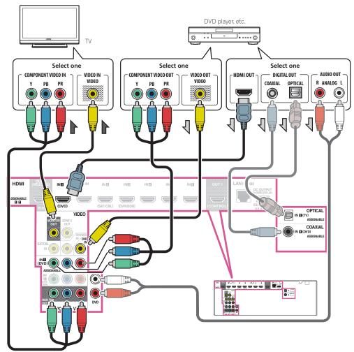
• In order to listening to HD audio with this receiver, connect an HDMI cable, and use analog video cable for video signal input.
