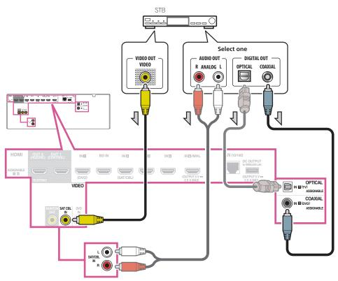
• With factory default settings, video from the video cable or component cable will not be output from the HDMI terminal. To output video, you must switch video input to the device connected with the video cable or component cable and set **V.CONV** to **ON** (page 69).
