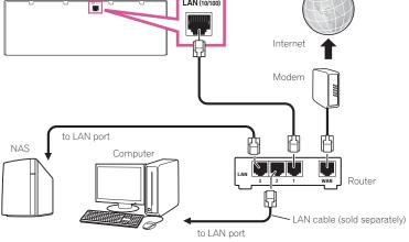
Connect the LAN terminal on this receiver to the LAN terminal on your router (with or without the built-in DHCP server function) with a straight LAN cable (CAT 5 or higher).
