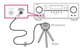
If you have a tripod, use it to place the microphone so that it's about ear level at your normal listening position. If you do not have a tripod, use some other object to install the microphone.
