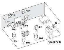
With these connections you can simultaneously enjoy 5.2-channel surround sound in the main zone with stereo playback of the same sound on the B speakers. The same connections also allow for 7.2-channel surround sound in the main zone when not using the B speakers.
