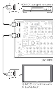
1 Use an HDMI cable to connect the HDMI IN 1/2 interconnect on this receiver to an HDMI output on your HDMI component.
