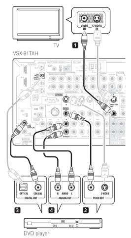
The diagram shows a basic setup of this receiver together with a TV and DVD player, with S-video or composite video connections. Different TVs and DVD players may offer alternative connections. See also *Using the component video jacks* on page 14 if your TV and/or DVD player has component video inputs/outputs. If your DVD player offers multichannel analog audio outputs, see *Connecting the multichannel analog inputs* on page 53.
