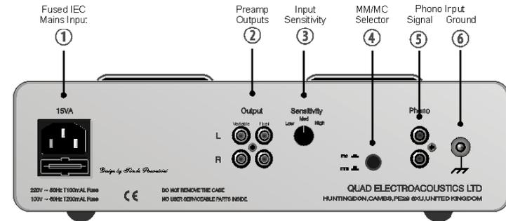
When making stereo connections to the QUAD *twenty four* P, RCA plugs and sockets coded *white* or *black* usually indicate the LEFT channel and those coded *red* the RIGHT channel. In a stereo pair of sockets the upper socket is usually the Left Channel and the lower socket the Right. If you are in any doubt, consult a qualified dealer.
