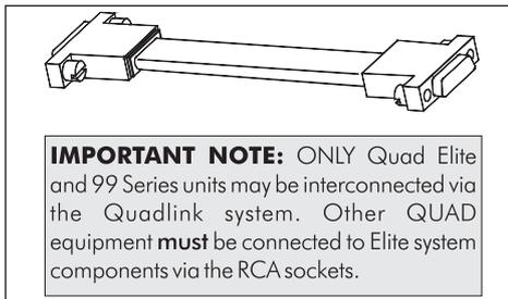
**IMPORTANT NOTE:** ONLY Quad Elite and 99 Series units may be interconnected via the Quadlink system. Other QUAD equipment **must** be connected to Elite system components via the RCA sockets.
