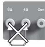
The QUAD II *eighty* has three output terminals – Common, 4 Ohms and 8 Ohms. Check the manufacturer's handbook for your speakers and use the terminal pair that most closely matches your speakers. Even though a loudspeaker may be rated at 8 Ohms or 4 Ohms its impedance varies with frequency – some experimentation may be necessary.
