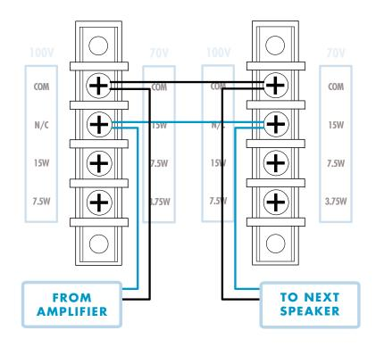
Select the power tap by dividing the amplifier's available power by the number of speakers to be connected and then selecting the next lower wattage tap. For example:
