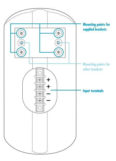
A complete installation kit designed to work with the supplied mounting brackets is included with each model and consists of:
