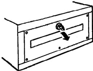
☛ Note: This lever is not a handle. When carrying the disc tray, always hold it by both edges.
