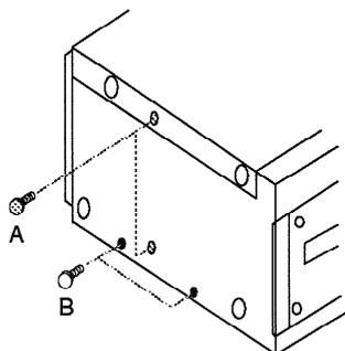
For superior rigidity and resistance against vibrations remove the two chassis locking screws [B] on each side of the CDC 100, so that the inner chassis floats inside the outer chassis.
