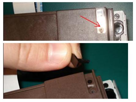
• Looking from the top, note the gear towards the front of the tray slightly right of center. Turn this gear clockwise until the pick-up and motor assembly drop to the load position.
