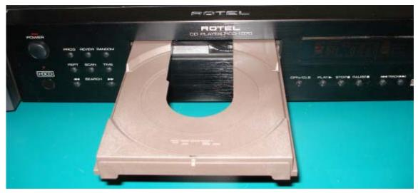
• Replace the cosmetic tray cover (see Step # 1). Ensure to slide the cosmetic tray cover down until both tabs "click" into place to ensure proper cosmetic alignment.
