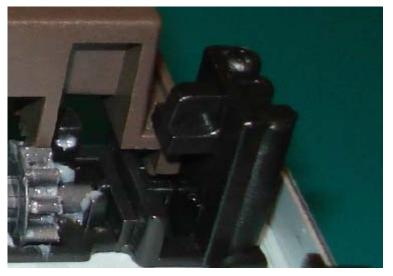
• Replace the locking pin and small screw using a #0 Phillips screwdriver.
