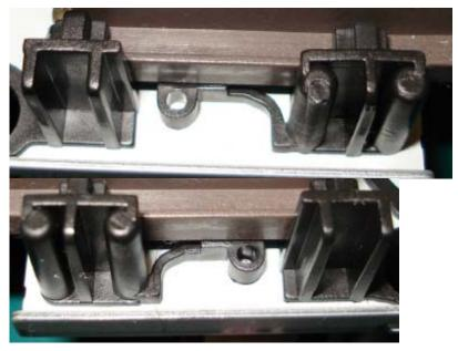
• Place your right thumb on the plastic cover towards the front of the mech and your right index finger on the back of the tray.
