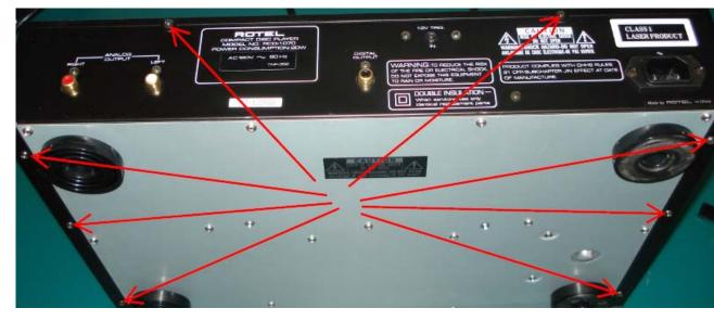
• Slide the top cover towards the back of the CD player and remove the top cover.
