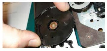
• Align the tray and insert it all the way into the mech.
