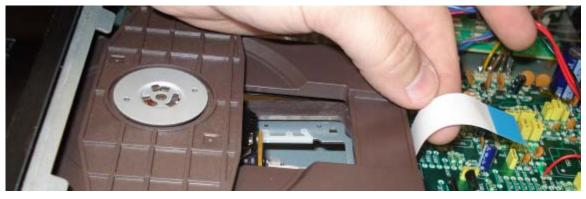
• Reconnect the two cables on the right of the mechanism to the main board.
