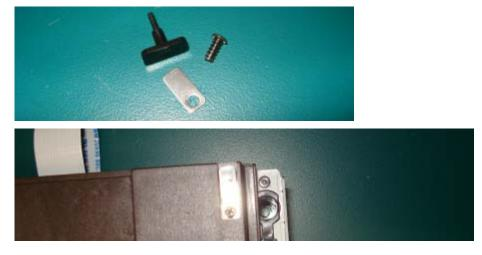
• Replace the disc clamper and secure with two small screws using a #1 Phillips screwdriver.
