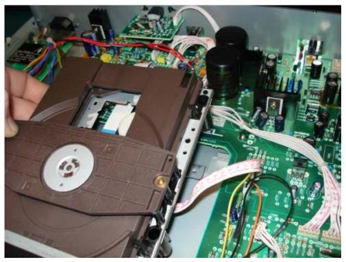
• Remove the mech from the chassis by lifting the rear of the mech above the main circuit board and sliding it towards the rear of the CD player.
