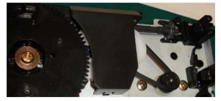
• Gently rotate the tray gear fully clockwise.
