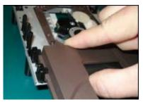
• Apply pressure to the back of the tray and using the Awl inserted into the small hole of the left retaining clip, gently move the retaining clip ¼ inch to the left (this will free the left side of the tray drawer).
