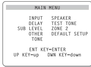
The MAIN menu provides access to nine other screens for various configuration options and is reached by pressing the ENTER button from the SYSTEM STATUS menu described above or from most other menus. To go to another menu, move the highlight to the desired line using the UP/DOWN buttons on the remote and press the ENTER button. Press the MENU key on the remote to cancel the display and return to normal operation.
