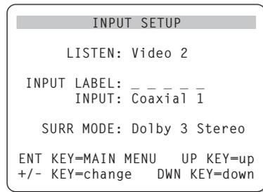
The INPUT SETUP menu configures the source inputs and is reached from the MAIN menu. The screen provides the following options, selected by placing the highlight on the desired line using the UP/DOWN buttons:
