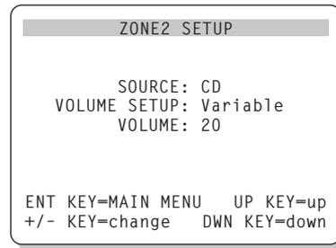
The ZONE 2 SETUP menu provides settings and configuration options related to the operation of Zone 2. This menu is reached by highlighting the ZONE 2 line on the MAIN menu and pressing ENTER.
