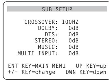
The SUBWOOFER SETUP menu allows selection of the subwoofer crossover frequency and independent adjustment of subwoofer level for each surround mode. These settings are memorized and engaged automatically each time a music or theater surround mode is selected.
