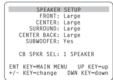
The SPEAKER SETUP menu is used to configure the RSX-1055 for use with your specific loudspeakers. The menu is accessed from the MAIN menu.
