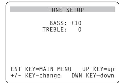
The TONE SETUP menu allows adjustment of the bass and treble settings.
