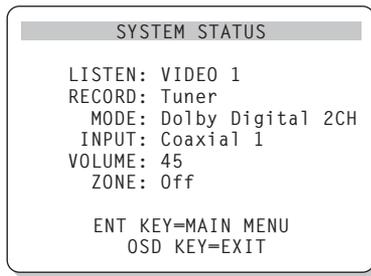
The SYSTEM STATUS menu provides a snapshot of the current system settings and a starting point for reaching all other screens and menus. This screen appears when you press the MENU button on the remote control and displays the following information:
