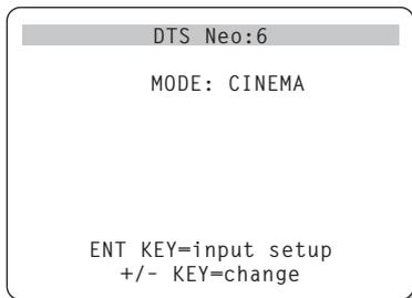
When Dolby Pro Logic II or DTS Neo:6 is selected as the default surround mode on the INPUT SETUP menu (see previous section), there are additional option settings and parameters available to optimize the surround decoding for various types of recordings, music or movie soundtracks.
