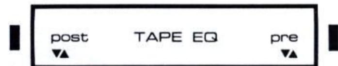
**Pre-TAPE-Post** — This switch determines how the equalizer will affect a tape deck or other component connected in the E101's tape loop. When the "pre" side is depressed, the LED lights and the equalizer is connected between the MAIN IN and the TAPE OUT. This provides the ability to modify your tapes as they are being recorded. This is particularly useful for car tapes or
