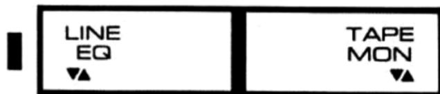
**LINE EQ** — Whenever this button is pushed, the EQ will modify the source (either main in or tape monitor) and will appear at the main output. (Remember, if "pre-TAPE" is selected, changing the parametric settings will affect the input to the tape deck.)
