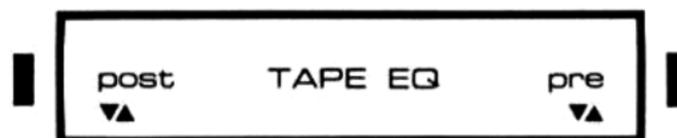
**Pre-TAPE-Post** — This switch determines how the equalizer will affect a tape deck or other component connected in the E101's tape loop. When the "pre" side is depressed, the LED lights and the equalizer is connected between the MAIN IN and the TAPE OUT. This provides the ability to modify your tapes as they are being recorded. This is particularly useful for car tapes or
