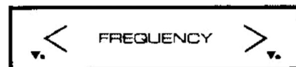
**FREQUENCY** — This control is used to determine the center frequency of the frequencies at which the EQ will take effect. The digital readout marked FREQUENCY displays this control setting and is
