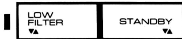
**LOW FILTER** — A special low-phase shift, low frequency filter is included in the E101. This filter should be engaged whenever acoustic feedback is noticed or when you have a high boost setting at low frequencies. (Below 40Hz.)
