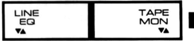
**TAPE MONITOR** — This switch provides access to the output of the tape loop. If you wish to listen to the tape recorder, simply depress this button. It will in no way affect the input to the tape deck.
