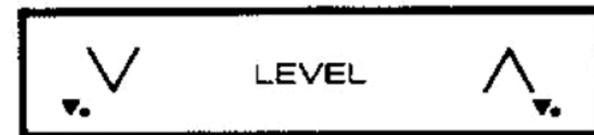
**LEVEL** — The level control determines the amount of boost or cut the control group will provide. Pressing the "▲" side will cause the signal to increase, while pressing the "▼" side will decrease the signal level. The actual level is indicated by the digital readout marked level in each control group. The display readout is in dB. (For further discussion see dB in the glossary.)
